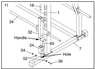
12. Place the Right Safety Spotter (23) on the right Base (7) and center it over the indicated hole. **Note: The handle must point toward the center of the bench.**
